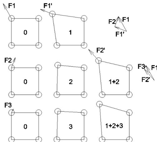
On each step, the residual force applied to the nodes and the displacement increment become smaller, leading to the convergence of the calculus.
